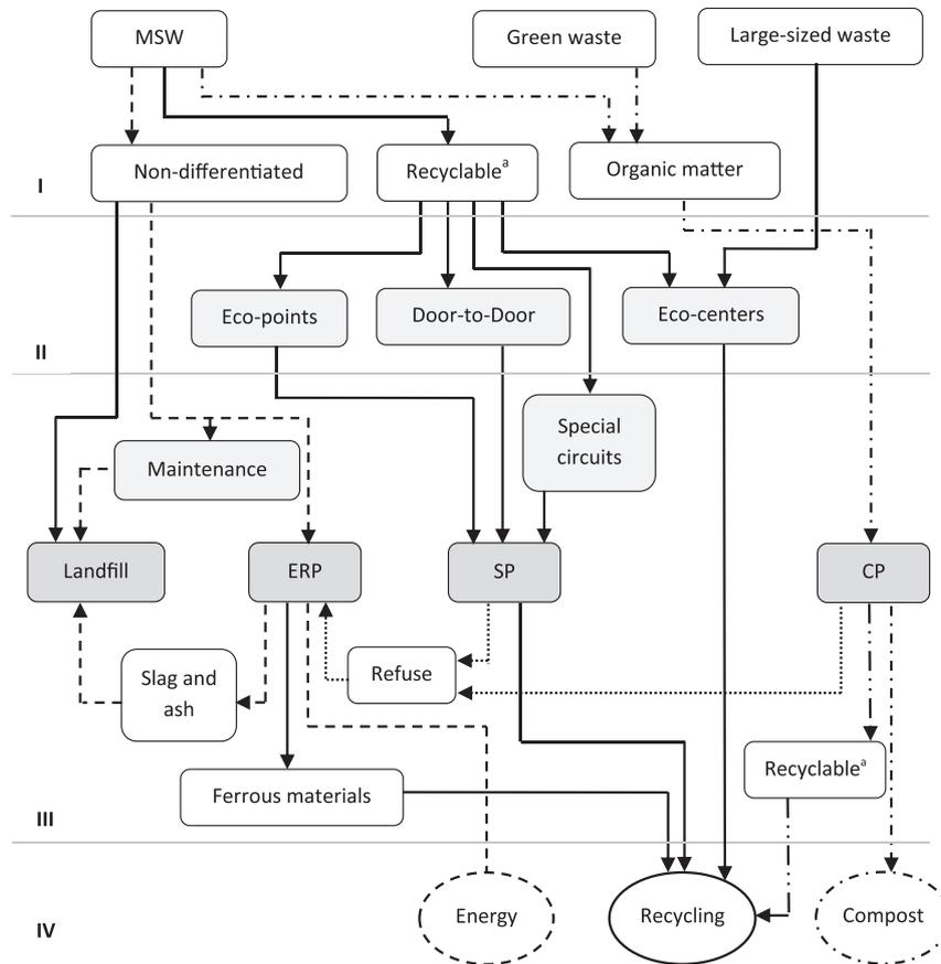
**Fig. 1.** The Integrated Waste Management System at LIPOR (adapted from LIPOR, 2009). ERP as the Energy Recovery Plant, SP as the Sorting Plant and CP as the Composting Plant. I – Citizen: production and disposal II – Councils: production and disposal III – LIPOR: valorization and treatment IV – Clients: products and resources <sup>a</sup> Recyclable are the wastes that can still be converted into valuable materials.
