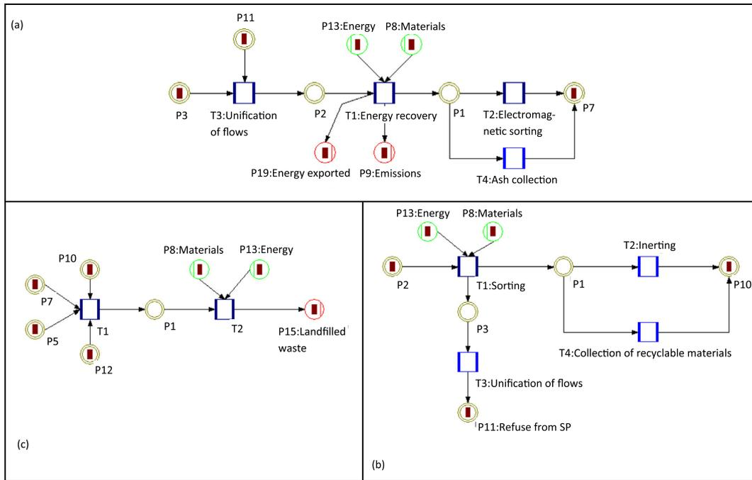
Fig. 4. Subnets from LIPOR's main network for 2010 modeled in Umberto®: (a) Energy Recovery Plant; (b) Sorting Plant; (c) Landfill.
