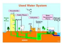
Figure 2. The Scheme of Used Water Management in Singapore [21].
