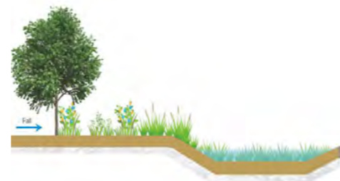
Fig.9.12 Vegetated Swale Source: ABC Water Guideline
